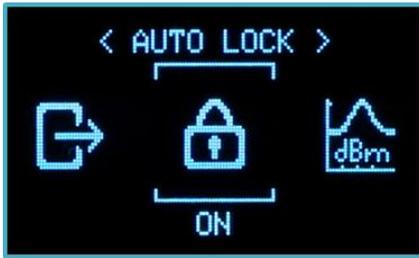
**Auto Lock:** To install **ON/OFF** in the setting menu. If you choose “**ON**” mode and exit to **Active Channel**, the main screen will auto lock after 10 seconds and cannot move by button. If you choose “**OFF**” mode, the screen will display continuously. By other way, at the “**Active Channel**” interface, hold **Select** button about 3s you can **Lock** and **Unlock** after press **Select** button once again.
