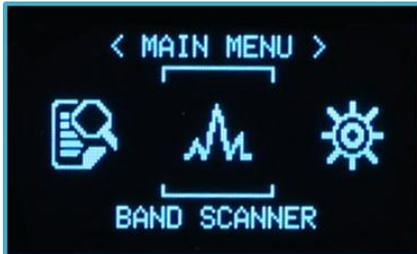
**Band Scanner:** Utilize to determine current broadcast band, channels and frequencies with a powered video transmitter. Identify a potential channel, band, and frequency with low noise for optimal use. Quickly find a pilot/VTX for spectating, troubleshooting, and even locating your lost drone by observing strength signal.
