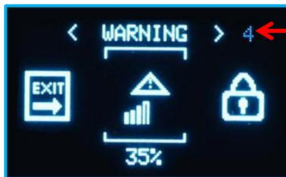
**Warning:** Buzzer will warn you at configured low signal level. The options are as follows: **None**, **20%**, **35%** and **50%**. If a low signal is detected on antenna A, the buzzer will single beep and if a low signal is detected on antenna B the buzzer will dual beep.
