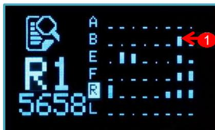
**Saved Channel:** To save channel that you want to choose to start up for the next time and delete undesired channel. When pressing the **Select** button about 3s, you can **save/delete/exit**. You can save up to 8 channels. **The default Saved Channels are R1 to R8.**
