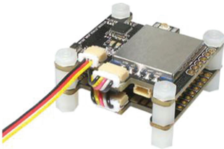
KOMBINI Flight Controller connect with PASSADO OSD-VTx
