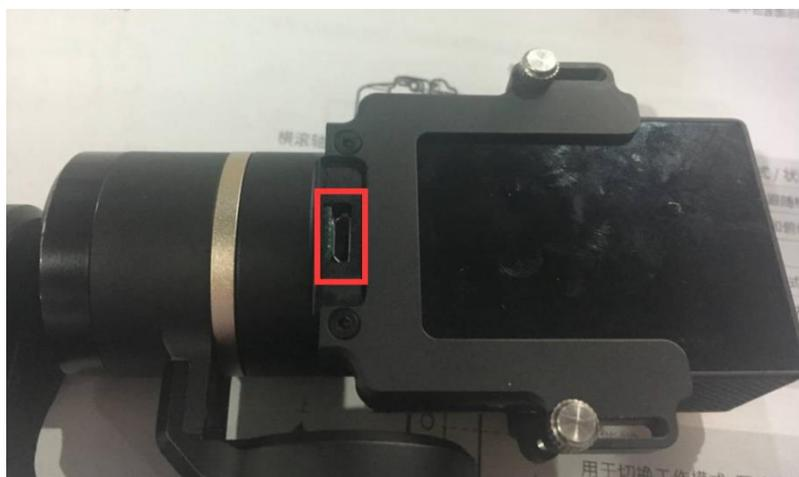
G5 can be used to charge with Gopro Hero series, the charging cables are Mini cable and Type C cable.
