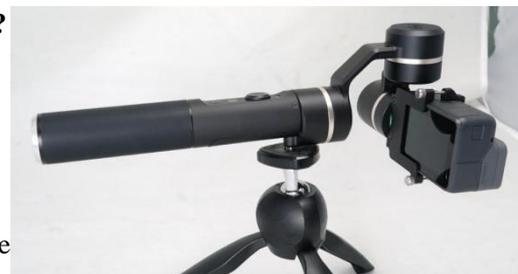
There is a M22 \* 1.5mm screw thread ON the bottom, It can be compatible with Feiyu extension bar.
