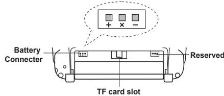
Pay attention to the battery connector polarity when connecting other batteries than the provided 6cell NiMH battery into the battery compartment, otherwise the Taranis X9D could not be powered on.
