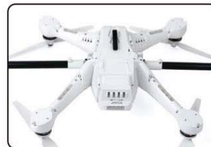
4.1.2 Turn X4 on its back. The belly and the retractable legs should now be facing up. MAKE SURE nothing is blocking the legs.
