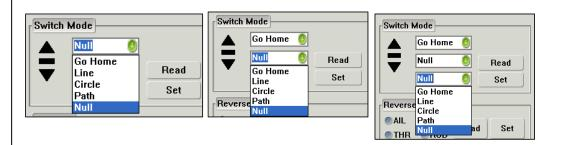
The Switch Mode setting allows you to select the function of each 3-Way switch position that controls the SW-2 channel.
